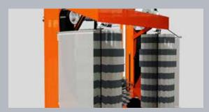
Micro-perforated curtains to prevent splashing during the wash process.
