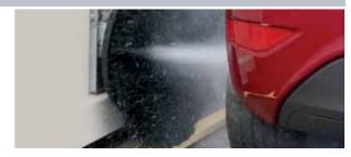
The new rotating 80 bar High Pressure fitted to the wheel wash means that the rims can be worked on more thoroughly as indeed can the whole vehicle itself. Its dual action spin gives better results on new wheel rim designs.
