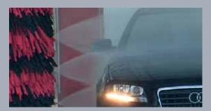
Various high pressure prewash options which prepare the vehicle for the brush wash and thus improve the results. Choose from versions: 15 bar and 120 l/min., 80 bar and 42 l/min. or 80 bar and 84 l/min.
